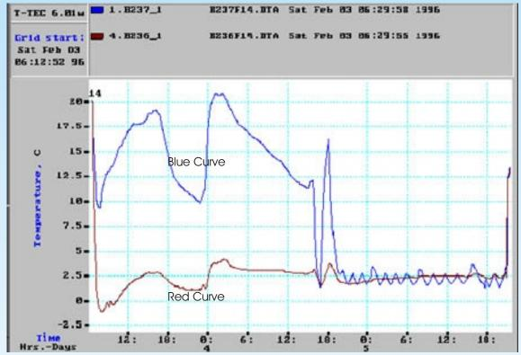
Example of a graph with 2 data loggers on a journey from Adelaide to Geneva with a shipment of fresh meat. The blue curve was a m b i e n t temperatures, the red curve was in the middle of the container.
